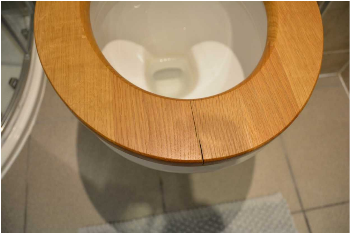
Crack in toilet seat.
